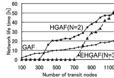
**Fig. 17** Network lifetime with various node density.
