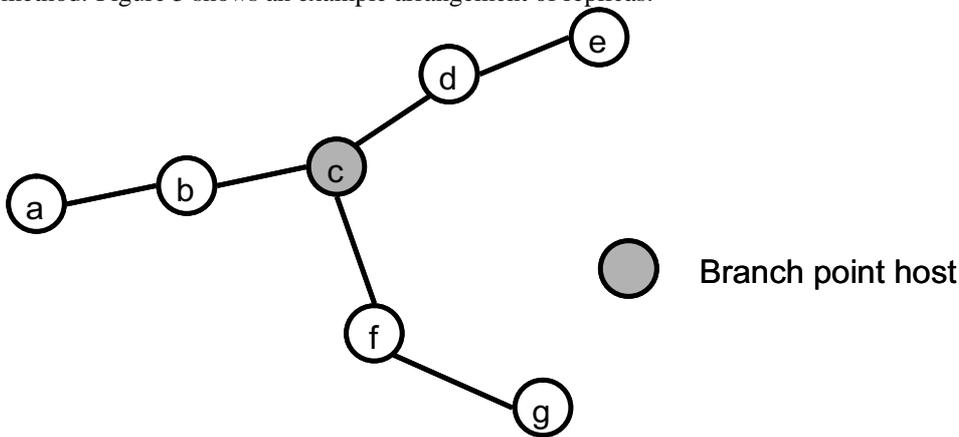
Figure 4 Branch point in ad hoc network
