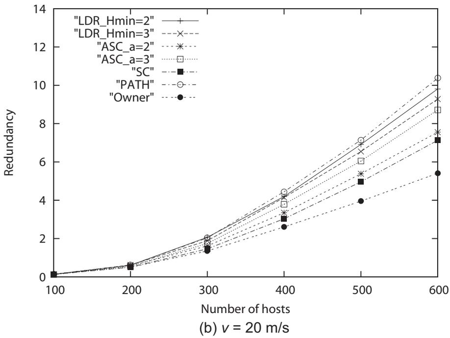
Figure 11 Redundancy vs. number of hosts (flat-priority model)
