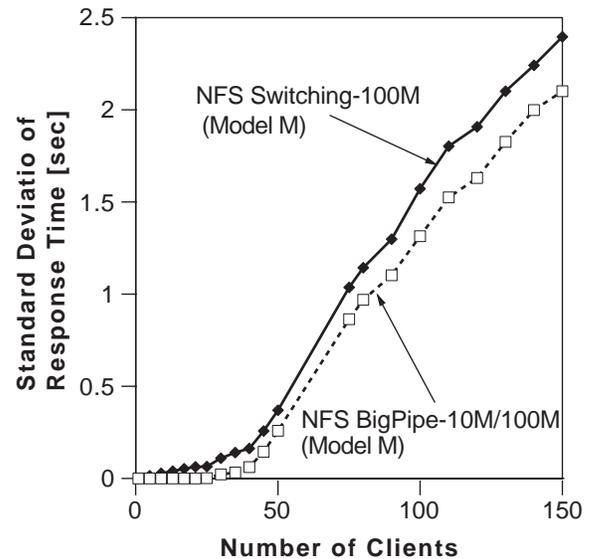
**Figure 7** Standard Deviation of Response Time (NFS Model M)
