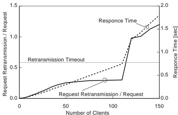
**Figure 5** Mean request time to a NFS request message and time-out of retransmission of NFS request. (Shared-10M Model M)
