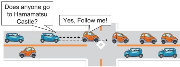
Figure 2: Query to neighboring vehicles which have smart blinkers
