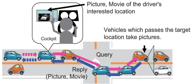
Figure 1: Live picture car navigation system
